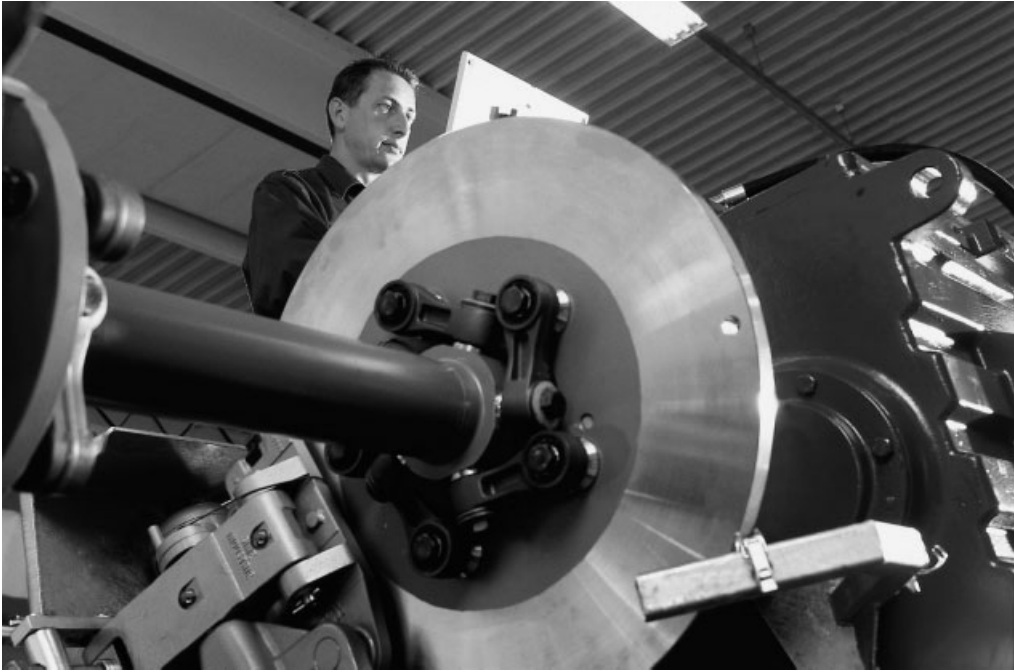
Figure 7.34 High-speed Shaft Brake Disc and Calliper (Reproduced by permission of NEG-Micon)
