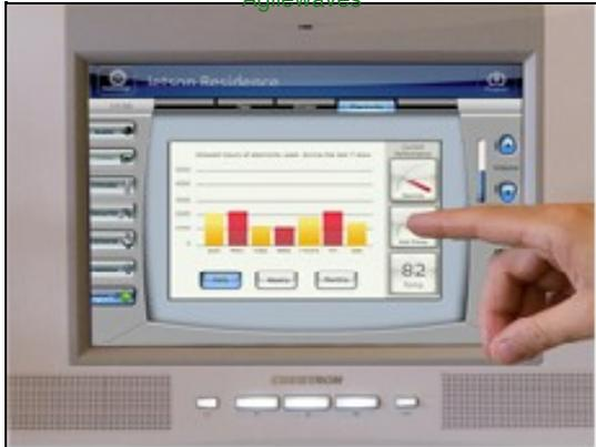
1. Agilewave's Resource Monitor tracks and manages energy consumption in real time from web-enabled devices.
