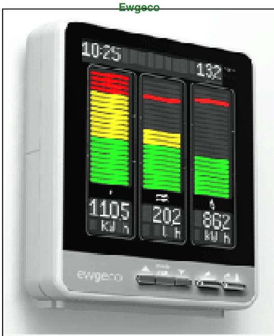
1. Ewgeco E200 displays overall electricity, and gas consumption.
