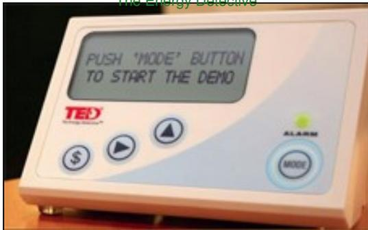
The Energy Detective (or TED) is one of the few energy management tools that allows to see electrical usage in real-time. TED quantifies electricity and displays the results on its easy-to-read LCD screen and/or a local or remote computer.
