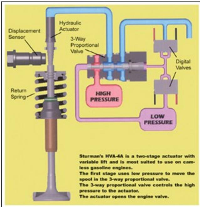
Hydraulically operated valve [Automotive Online](http://AutomotiveOnline.com)
